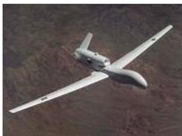
Figure 7: RQ-4 Global Hawk unmanned aerial vehicle
